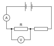
The reading on the ammeter is 2.0 A and the reading on the voltmeter is 8.0 V.
